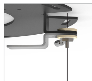
6. Insert the 4 wires through the 4 wire grippers.
