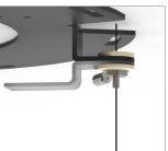
6. Insert the 3 wires through the 3 wire grippers.
