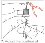
the lamp and then cut the excess of wire. Wires can't touch anything.
