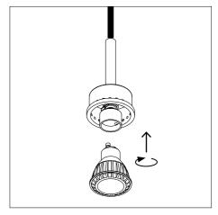
2. Place the GU10 light bulb in the socket as illustrated. **Not included:** GU10 light bulb
