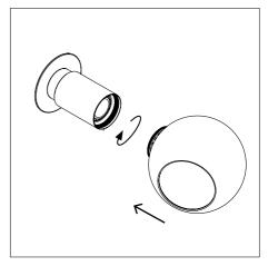
**4.** Screw the glass shade with the base. Fixate it by turning the glass shade clockwise.
