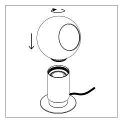
3. Attach the glass shade to the cylinder as illustrated. Fixate it by turning the glass shade clockwise. Turn it all the way in.
