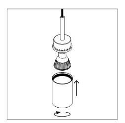
3. Connect the cylinder with the base as illustrated. Fixate it by turning it all the way clockwise.
