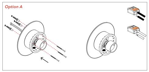
**1A.** Mount the lamp base to the wall with 3 wall screws and 3 wall plugs. Please make sure it is attached securely to the wall.
