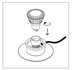
1. Place the GU10 light bulb in the socket.
