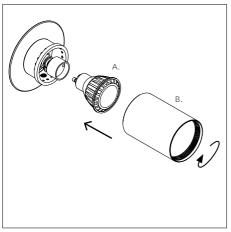
**3.** Place the Gu10 light bulb in the socket. Then, screw the metal tube with the base. Fixate it by turning te tube clockwise.
