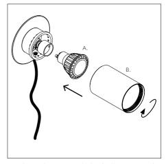
2. Place the GU10 light bulb (A.) in the socket. Then, connect the cylinder (B.) with the base. Fixate it by turning the cylinder all the way in, clockwise. **Not included:** GU10 light bulb
