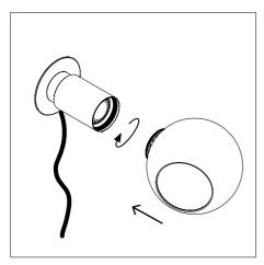
3. Attach the glass shade to the cylinder as illustrated. Fixate it by turning the glass shade clockwise. Turn it all the way in.
