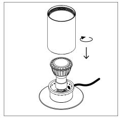
2. Connect the cylinder with the base as illustrated. Fixate it by turning it all the way clockwise. **Not included:** GU10 light bulb
