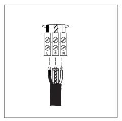
1. Adjust the length of the textile cable to fit your requirements. Lead the textile cable into the cable connector.
