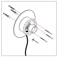
1. Mount the lamp base to the wall with 3 screws and 3 wall plugs. Please make sure it is attached securely to the wall.
