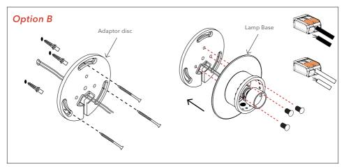
**1B.** Select and employ screw anchors, which are suited to the surface where the appliance is to be installed. Mount the adaptor disc to the wall with 3 wall screws.
