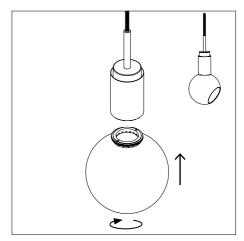
4. Attach the glass shade to the cylinder as illustrated. Fixate it by turning the glass shade clockwise. Turn it all the way in.
