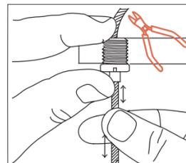
7. Adjust the position of the lamp and then cut the excess of wire. Wires can't touch anything.
