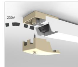
8. Connect the primary power cable to the terminals on the primary side of the power supply and then, fasten the screw of the safety cap.
