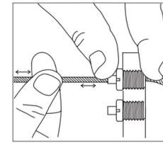
7. Adjust the height of the lamp by pressing the wire gripper and then, cut the excess wire, as shown.
