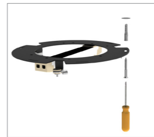
2. Drill 5 holes, place the anchors and fasten the ceiling bracket. Make sure it is equally fixed.
