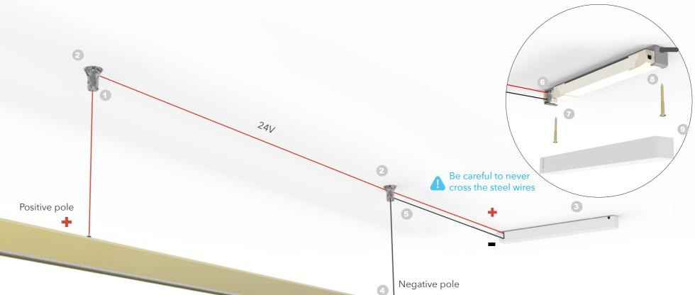
4. Insert the steel wires
